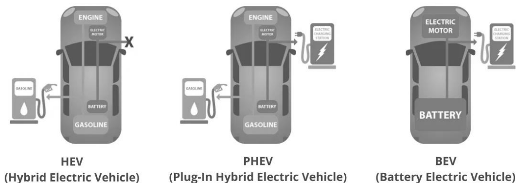
Figure 1. Comparison of electric vehicle types: Hybrid Electric Vehicles (HEVs); Plug-in Hybrid Electric Vehicles (PHEVs) and Battery Electric Vehicles (BEVs).
